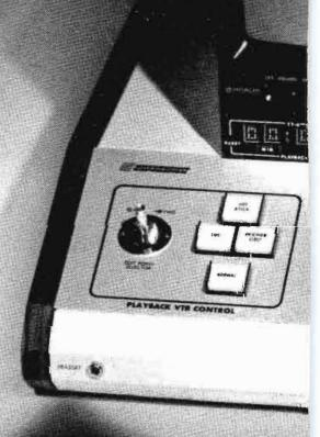
SM-2 Joystick Search Module gives you incredibly flexible tape handling and remote control on a stand-alone VCR. The unique Convergence joystick allows you to see pictures at speeds continuously variable from still frame to three times normal play in forward and reverse. The LED tape timer lets you quickly screen and log news stories or commercials for pre-edit decision making. The SM-2 also programs precise on-air roll cues and lets you slave extra playback machines for A/B rolls.
