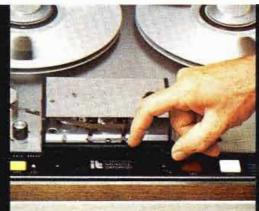
"When I touch FAST, the gate opens automatically and lifts the tape from the head. Or, I can open the gate manually. Manual positioning, or 'gating', lets me monitor the tape in high speed modes without risking damage to meter, amplifiers or speakers."
