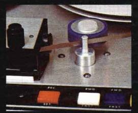
"This new high-friction polyeurethane roller pulls the tape with less pressure. Less wow and flutter."
