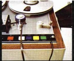
"Dumping tape in the edit mode is fast, easy, foolproof. Moving the tension arm down turns the take-up reel off. I can discard tape, listening as I go."
